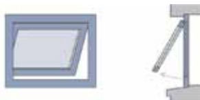
Top hung casement, outward opening
