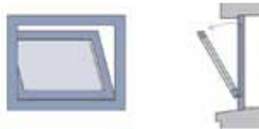
Bottom hung casement, outward opening
