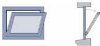
Bottom hung casement, inward opening
