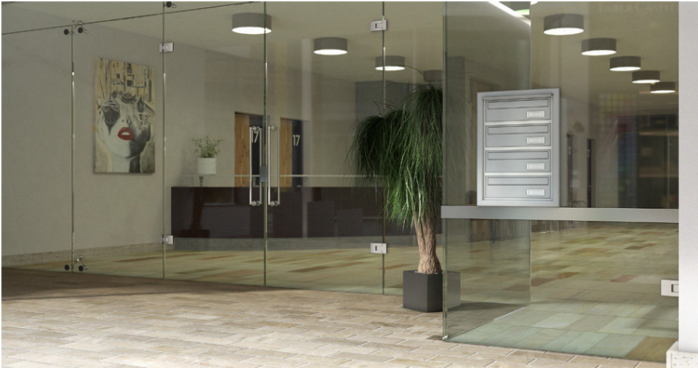
Casellare postale incassato su serramento composto da cassette SC6 e completo di mantello, profilo coprifuga e sgocciolatoio. Recessed fixture-mounted modular letterbox unit consisting of model SC6 letterboxes and inclusive of shell, gap covering profile and drip profile.
