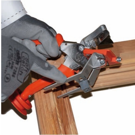
Fit the frame accessory onto the cutter
