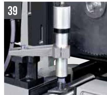
TIGER 352MA/COBRA 352MA Pneumatic vertical vice
