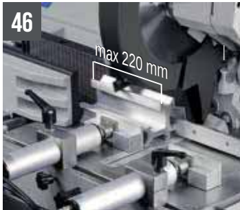
46 COBRA 352 NC 5.0 Special vice to reduce restpiece
