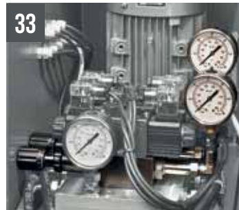
SHARK NC 5.0 Hydraulic vice pressure adjuster
