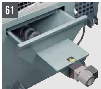
SHARK 230-1 / 331-1 NC 5.0 spider Powered chip auger
