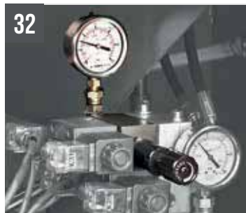
SHARK SXI evo Hydraulic vice pressure adjuster
