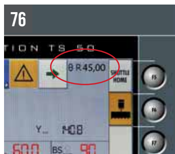
SHARK 332-1 NC 5.0 Digital Angle Display
