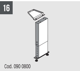
SHARK 281 SXI evo Adapter for unloading table
