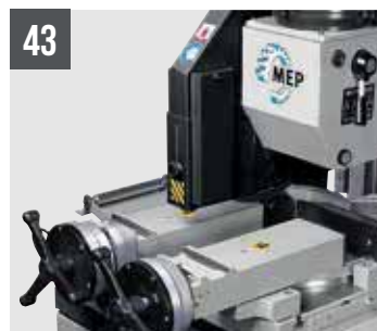
TIGER 352MA/SXevo/NC 5.0 TIGER 372 SXevo Supplementary pneumatic vice
