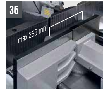
SHARK 332-1 NC 5.0 Special vice to reduce restpiece
