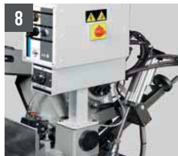
SHARK 282 Cut Control System (kit to retrofit)
