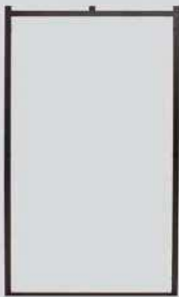
2 Leaves door frame - upper gap 40 mm - upper horizontal profile 40x30mm with central support - lower horizontal profile 20x30mm
