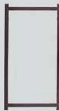
1 Leaf window frame -upper gap 40mm -upper and lower horizontal profiles 40x30mm - lower gap 40mm
